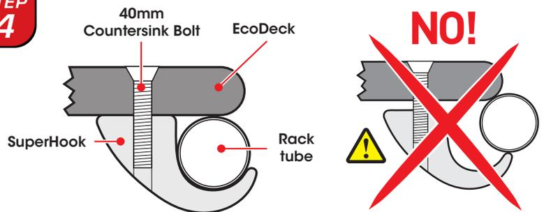
Place EcoDeck with SuperHooks on top of racks. Install one side at a time. Twist SuperHooks so that they are aligned with and snug to racks. Once SuperHooks are in proper place, tighten one side until firmly secure. With one side complete, repeat on other side. If the rack distance is too wide, refer to **Step 2** above to squeeze them together until SuperHooks are completely under the rack. Tighten SuperHooks bolts and remove CamStrap or belt when finished. **DO NOT pinch rack with SuperHook**
