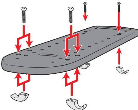
Install the four countersink bolts into the EcoDeck's countersunk holes. Screw bolts into SuperHooks a couple turns so that **they're on, but loose**. The forward hook positions have two options for install, but we recommend using the forward most holes.
