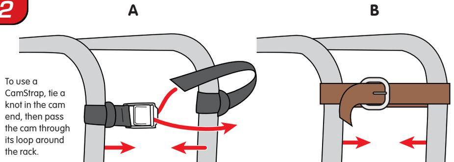
To use a CamStrap, tie a knot in the cam end, then pass the cam through its loop around the rack.
